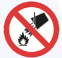
Do not extinguish with water
